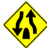
Divided Roadway Ends
